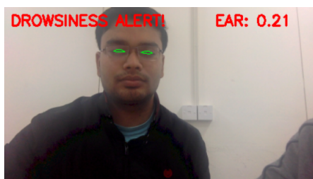
Figure 14: A team member being warned of drowsiness using our eye detection system on April 3, 2018
