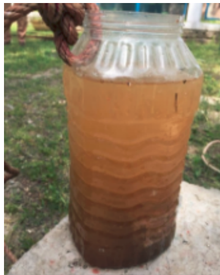
Figure 6: Water sample from a closed tap, showing possible iron contamination
