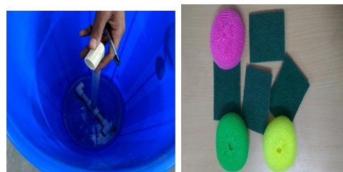
(a) Inlet Pipe (b) Scrubber layer of bio filter
