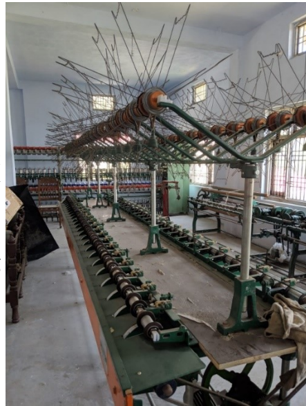
Fig. 3: Modern reeling machine (Vadivazhagu, 2019).
